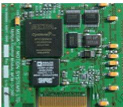
The control power of MC-804 Controller is based on the core module MAC-204, which is a 4-axis member of Mega-Fabs family of Multi-Axis Control modules [MAC-2xx](#). (This module plugged in the MC-804 controller is outlined by red on the front page picture).
